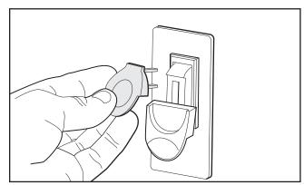
**Figure 11.** Removing switch key from paddle switch.
